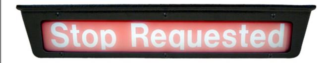
Transign Stop Requested signs are used internationally to communicate when a passenger has used the next stop request system, and have been considered an industry standard for nearly 60 years. These high quality signs can also convey messages to departing passengers for safety or wayfinding purposes, and are available in multiple languages.
